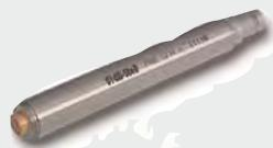
The type 26AA, 26AB, 26AC and 26AL 1/4" preamplifiers are small rugged units optimized for acoustical measurements with condenser microphones. They have a very low inherent noise level, a wide dynamic range and a frequency range from below 2 Hz to above 200 kHz. Type 26CB 1/4" ICP® preamplifier with standard BNC output connector is intended for use with pre-polarized microphones. Special 1/4" to 1/2" adapter is available to use with 1/2" microphones.
